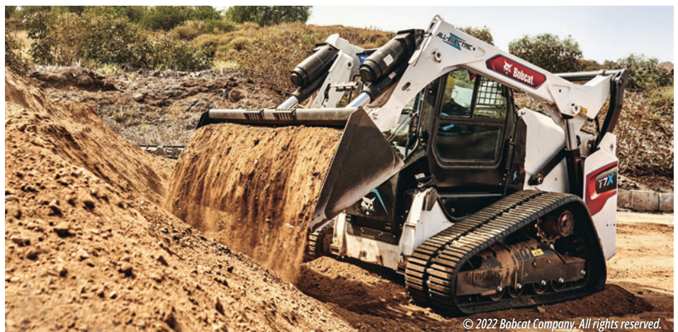
Bobcat® T7X All-Electric Compact Truck Loader, Moog Intelligent Electrification System Courtesy of Bobcat Company
