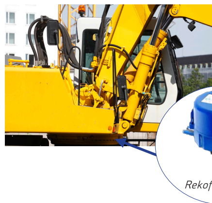
Figure 1: Slip ring for power and signals
